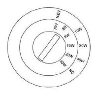
For easy adjustment of the tap settings With options for: 5W, 10W, 20W, 40W (70V) 10W, 20W, 40W, NC (100V)  $8\Omega$  Bypass
